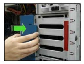
4. Secure the fan cage with the thumb screw.
